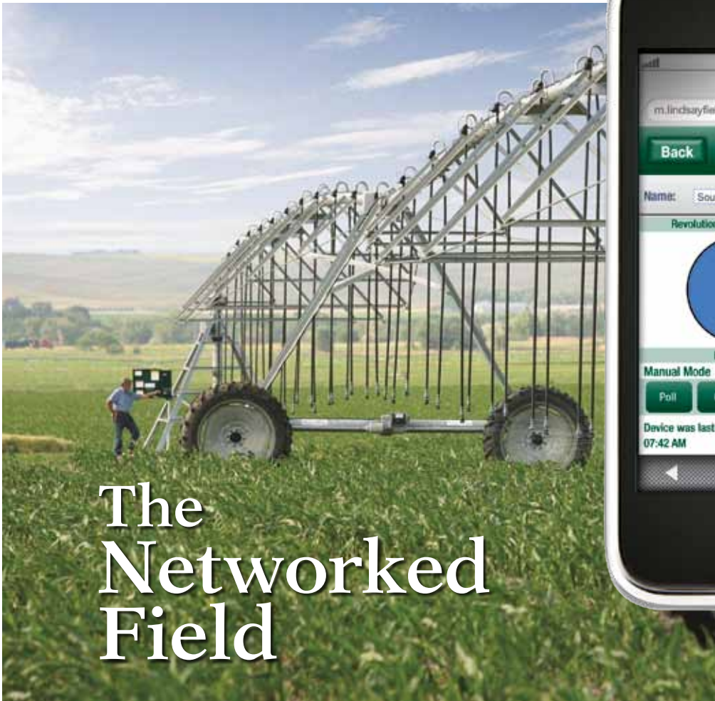
A screen capture shows Lindsay Corporation's mobile app that allows farmers to control irrigation pivots from anywhere in the field.
